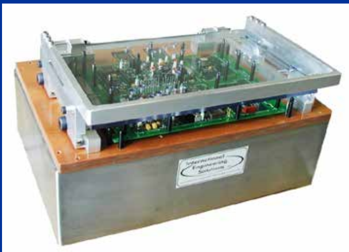
Functional Automated Test System: Functionally tests loaded PC boards using a typical bed of nails fixture pictured below.
