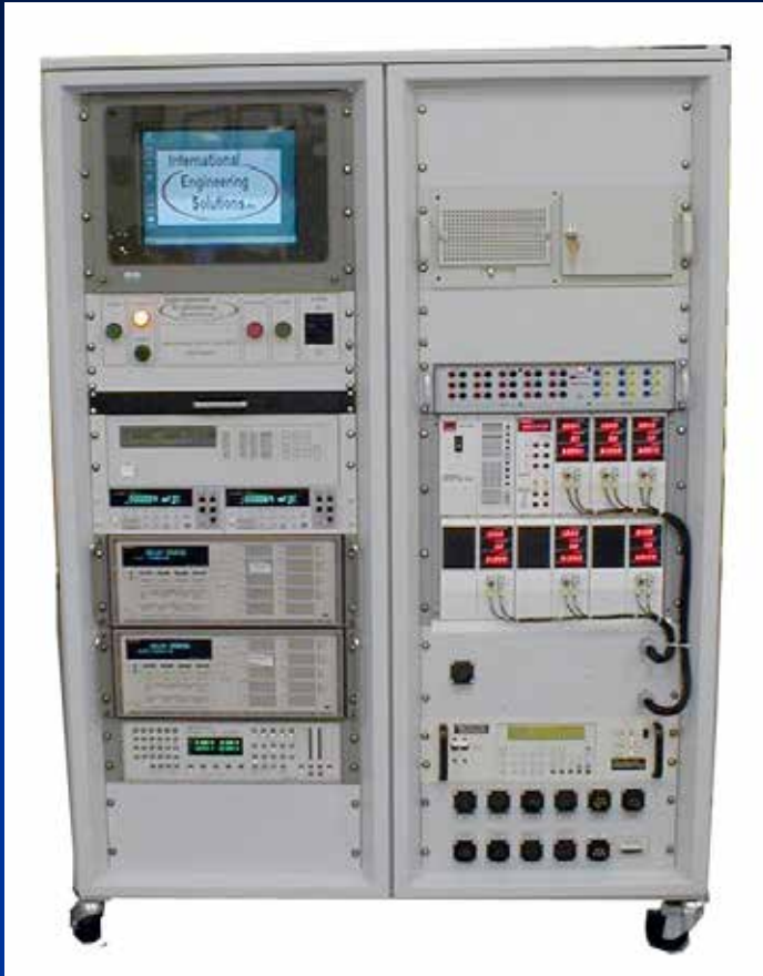
Functional Automated Test System: Functionally tests loaded PC boards using a typical bed of nails fixture pictured below.
